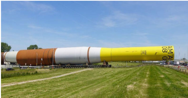
Figure 5: Transport of a monopile on SPMT
